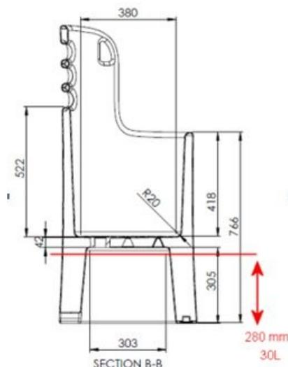
To stabilize the product, max 30 liters of water is added into the bottom tank. The water-filling hole is in the bottom. The water needs to be added when the product is in a horizontal position. We recommend you change the water once a year. There is a 3-mm vent hole in the upper corner.
