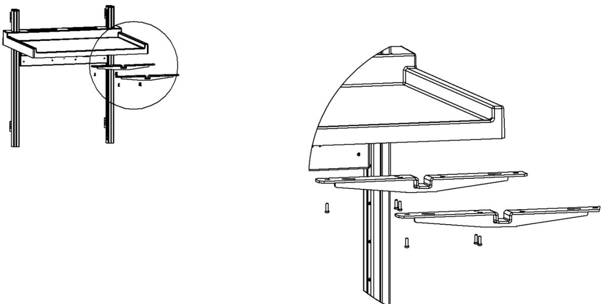
d) Mount the two fixing bolts between the tops
