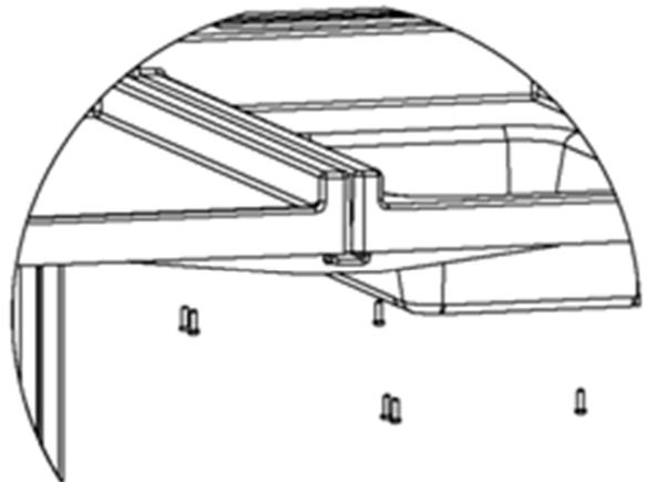
The crack between the two tops can be sealed with sealant. Be sure to clean the surface with a gentle household cleanser prior to sealing. Tops are made of ABS.
