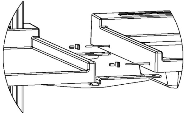
e) Finish by mounting two support brackets on the side sink
