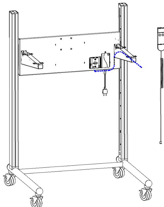
d) Mount top in pre drilled holes
