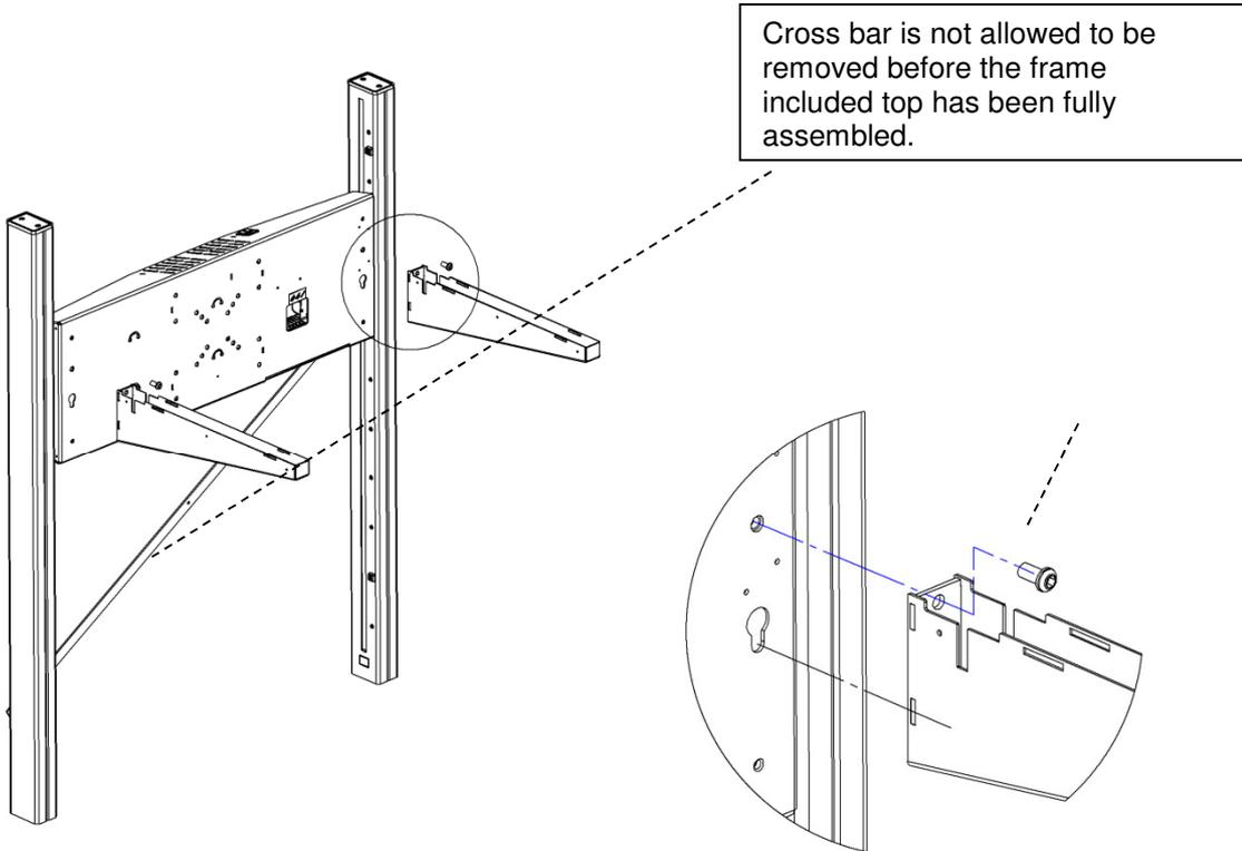
b) Mount four fixing brackets for top and attach three lead holders with screws.
