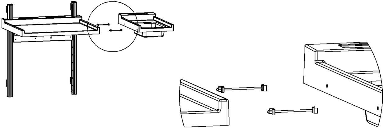
b) Make two  $\varnothing 8$  mm holes in both top and sink as shown in drawing. Holes to be used with the fixing bolts.
