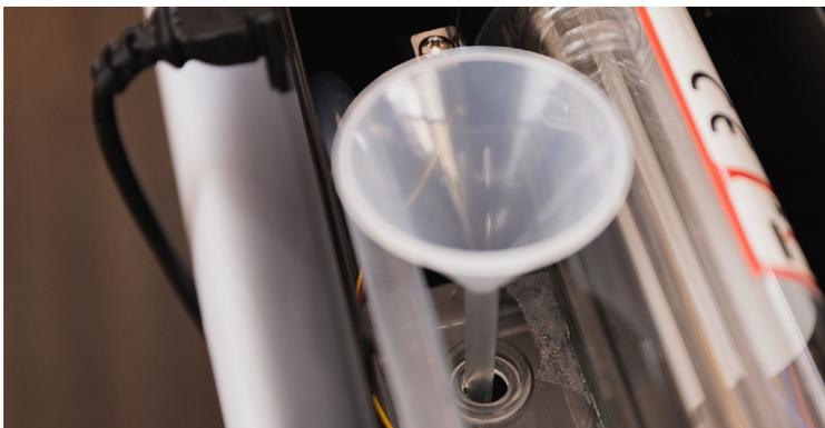
▲ Fill up the tank using a funnel. Watch the water level carefully to prevent from spilling over
