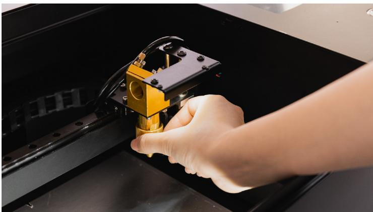
▲ Release and remove the lens holder.
