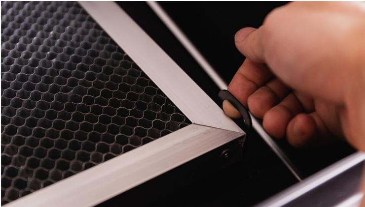
2 Use vacuum cleaner or brush to clear the left-overs bits under the tray. Detergent can be applied to remove the stains.
