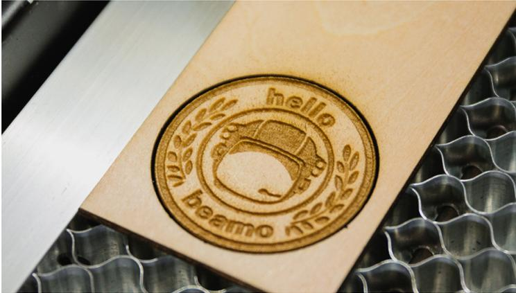
If the result is too light or blurry, please check if the focus is just right. If the focus is right but the result is poor, please recheck the optical path. See "Optical Path Adjustment" (p.60). If the position of the result varies with the camera preview, please recheck the focus or see "Camera Alignment Issue" (p.95).
