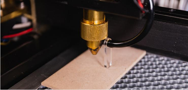
▲ The probe should precisely touches the surface of the material
