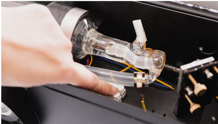
4 Remove the screws of the laser tube holder on both sides.
