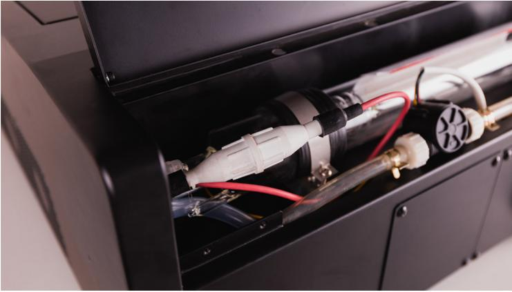
▲ Reconnect the connector on the high-voltage side
