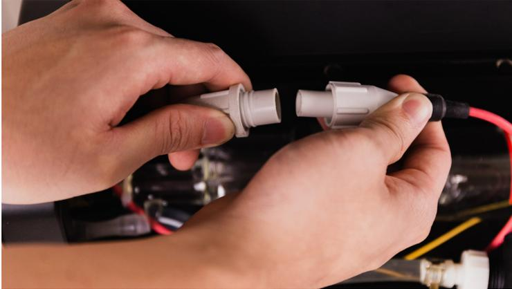
3 Find the white terminal near the low-voltage side. Press the button on the white terminal to release and remove the cable connected to the low voltage side.
