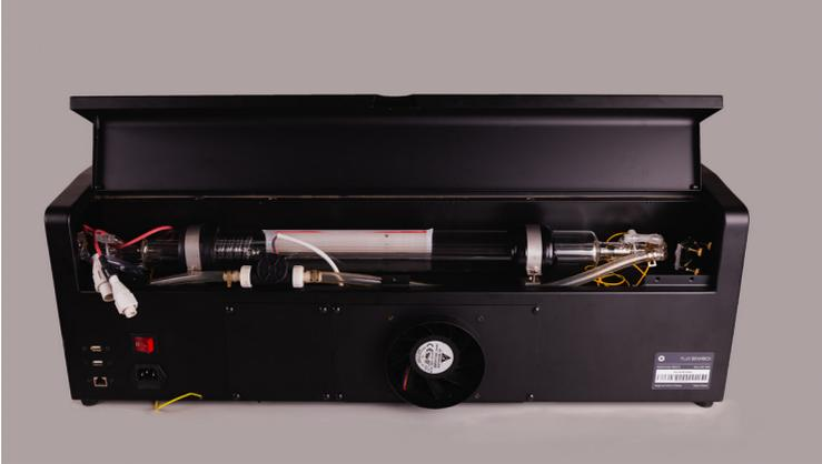
▲ Place the new laser tube and connect the hoses
