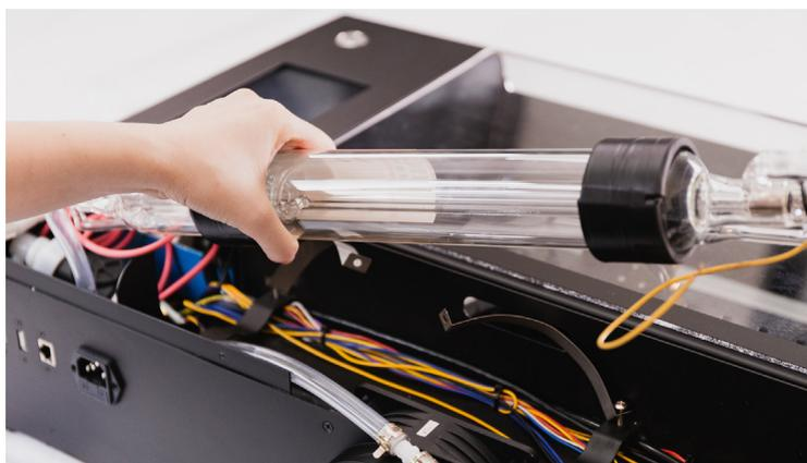
▲ The laser tube can be entirely removed
