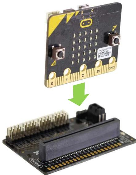
**Inserting a BBC micro:bit:** To use the servo driver board the BBC micro:bit should be inserted firmly into the connector as shown left.
