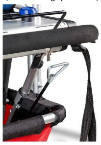
If the E-Turtle Kiddy Bus has to be driven manually, the motor is set to freewheel by means of the handle under the push handle. If the handle is pulled upwards and held against the push handle, the vehicle can be driven manually. When the handle is released, the motor is re-coupled by means of a spring.
