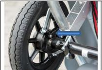
Lubricate the tilting arm on both rear wheels at least once a year.
