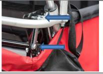
3) Lubricate the P-brake once a year on both sides, top and bottom.
