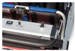
The ignition key switches the power on and off: Turn to the right to switch on. Turn left to switch off.
